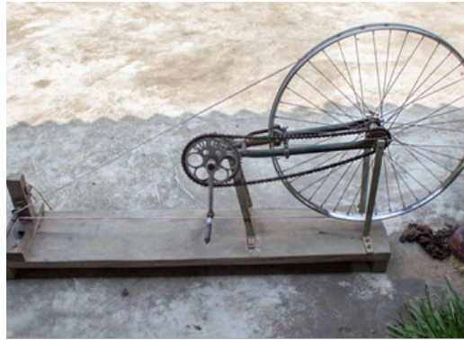
The manual spinning wheel is used to wind yarn on a small wooden stick.
