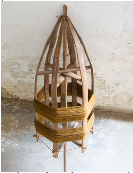
Winder is used to wind yarn appropriately
