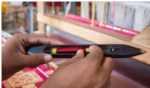
Pirn is placed in the flying shuttle for weft process.
