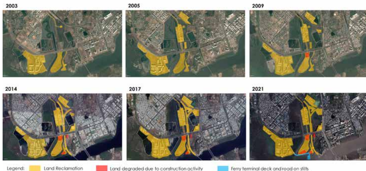
Figure 5: Expansion of reclaimed land and loss of mangroves from 2003 to 2021 (Source: Adapted by author from Google Earth)
